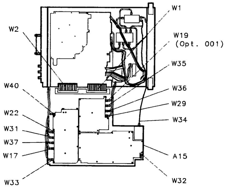
**Figure 5-5. Bottom View (A15 Unfolded)**
