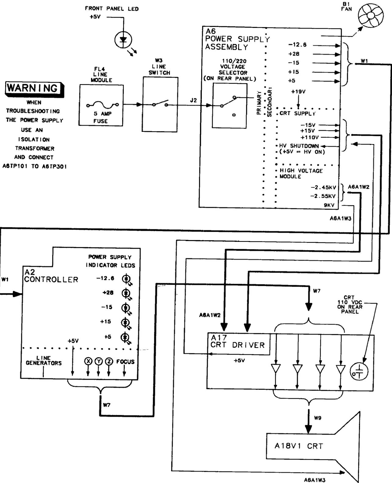
Figure 13-1. Simplified Section Block Diagram
