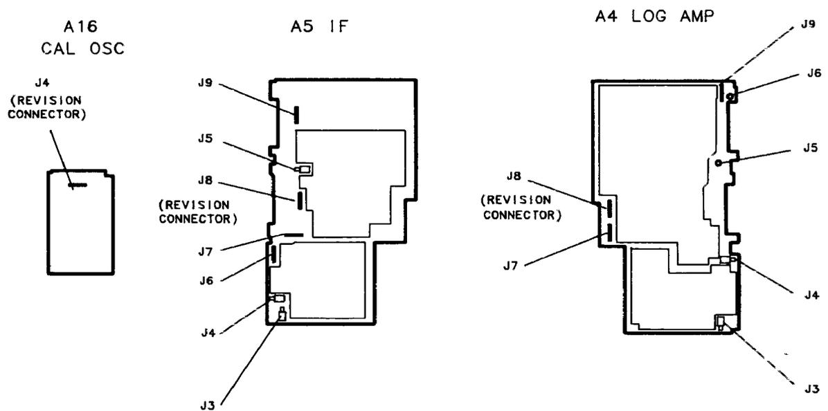
Figure 9-1. A4, A5, and A16 Test Connectors
