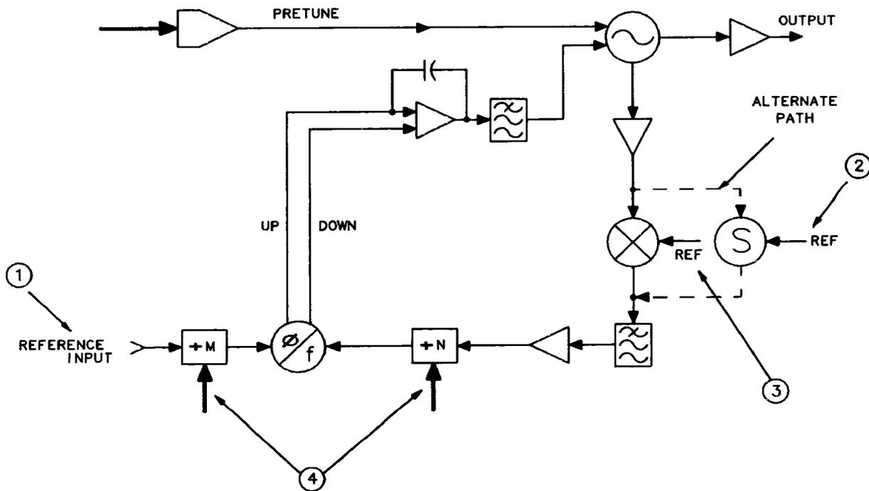
Figure 11-4. PLL Locked at Wrong Frequency
