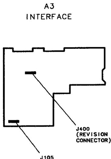
**Figure 8-1. A3 Test Connectors**
