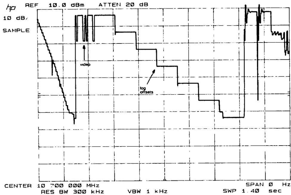
Figure 9-7. Detailed IF Adjust Signature (4)
