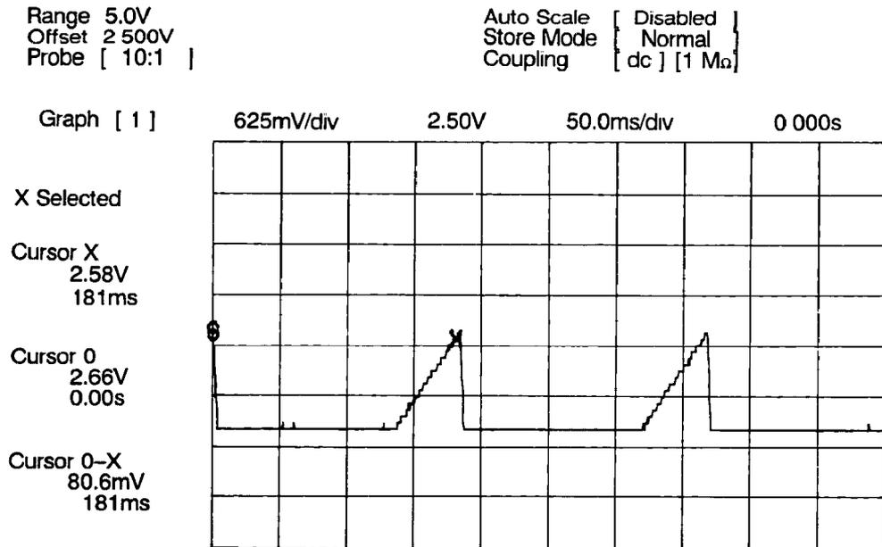
**Figure 12-4. Signal at A14J15 Pin 1**
