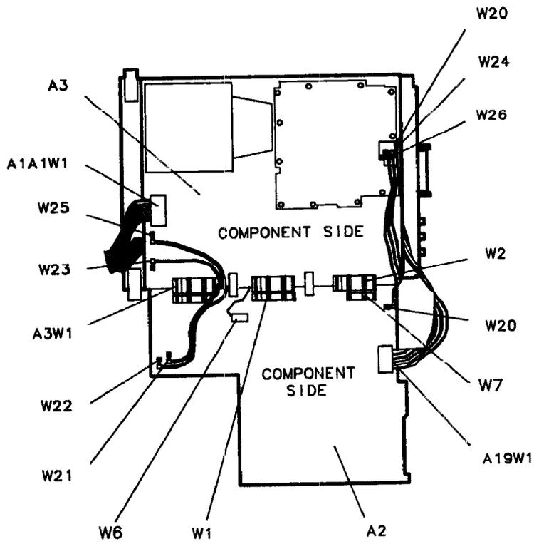
**Figure 5-2. Top View (A2 Unfolded)**
