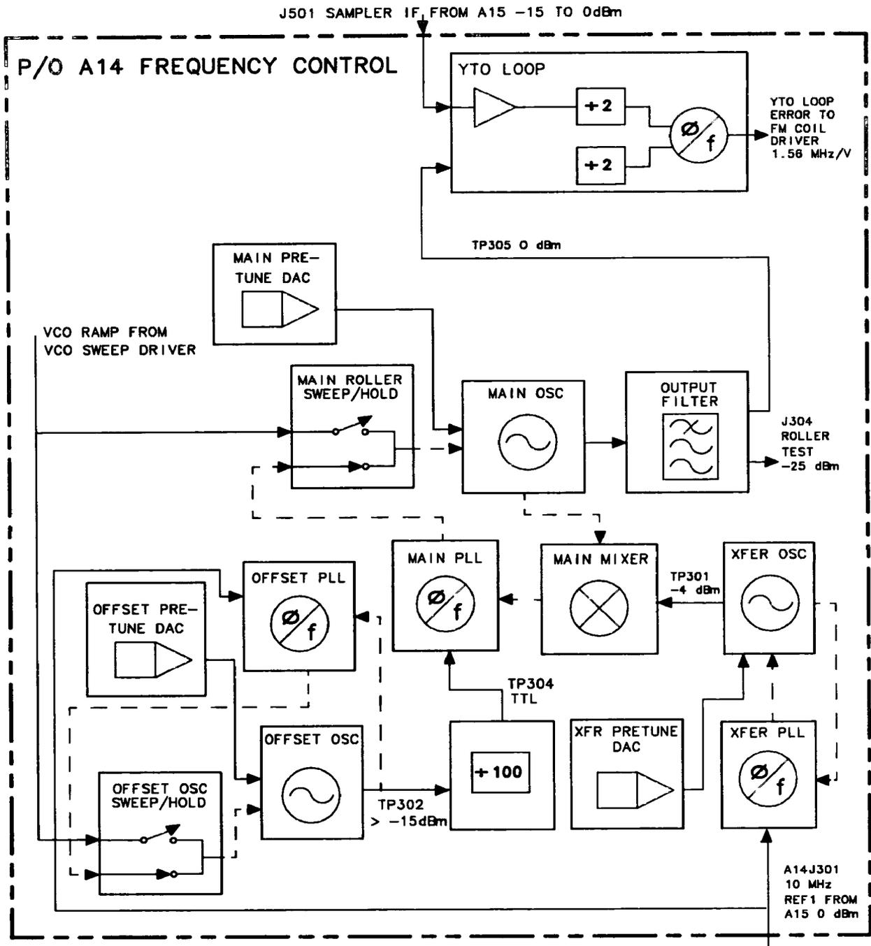
Figure 11-13. Simplified A14 Assembly Block Diagram
