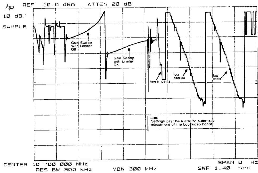
Figure 9-6. Detailed IF Adjust Signature (3)
