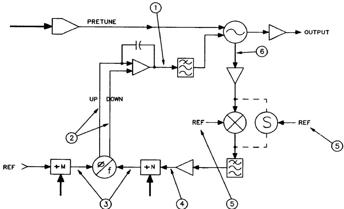
Figure 11-5. Unlocked PLL
