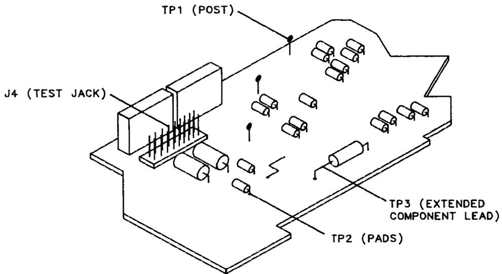
Figure 7-1. Assembly Test Points
