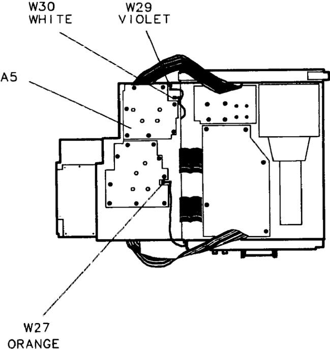
Figure 3-9. Assembly Cables (2 of 2)
