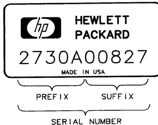
Figure 1-1. Typical Serial Number Label
