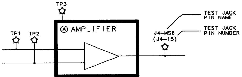
TEST POINTS ON CIRCUIT BOARD ASSEMBLY
