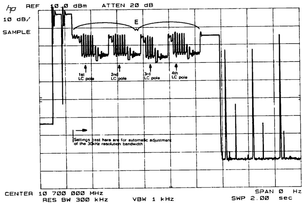
Figure 9-8. Detailed IF Adjust Signature (5)
