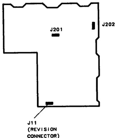
**Figure 10-1. A2 Test Connectors**
