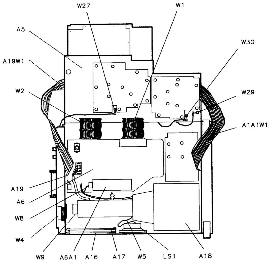
**Figure 5-4. Top View (A2, A3, A4, and A5 Unfolded)**
